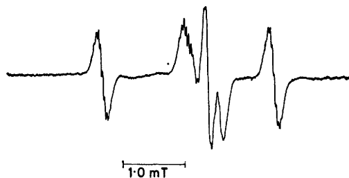
FIGURE 2 E.s.r. spectrum from 2,4,6-trichloronitrosobenzene and 2,4,6-tri- t -butylphenol 45 min after admixture. The asymmetrical centre shows the waning initial signal of the 2,4,6- t -butylphenoxy radical
